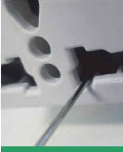
Fig 3. Access to live parts
