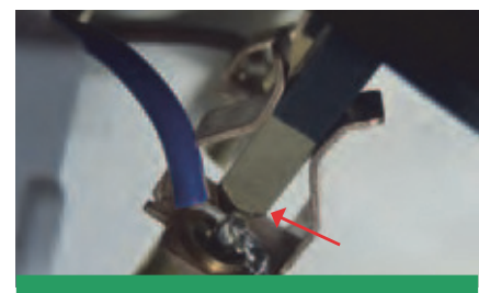
Fig 2. Soldered connections in the accessory prevented the test plug being fully inserted
